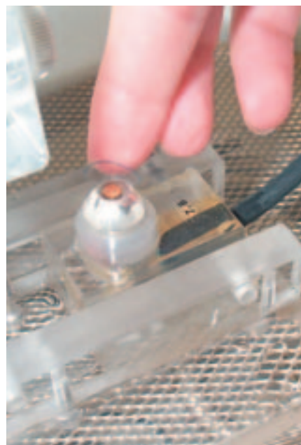
FIGURE 4. Draping a soft lens over a polarographic electrode for the measurement of oxygen performance
